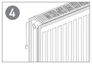
Place the magnetic temperature sensor between the radiator plates on the supply side (the side with the knob). Connect the power adapter to the nearest socket. The Comfort is now ready for use.
